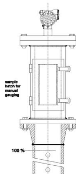
*Good results are obtained using so called 'hinged door' constructions. A hinged door access can be used for both servo and radar technologies.*
