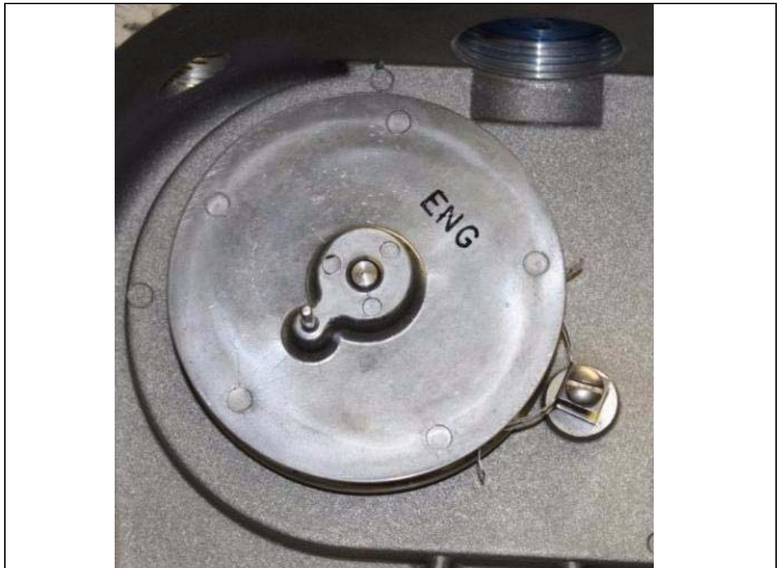
Figure 3-2: Pin Drive at 8 o'clock on the Sprocket Sheave Diagram
